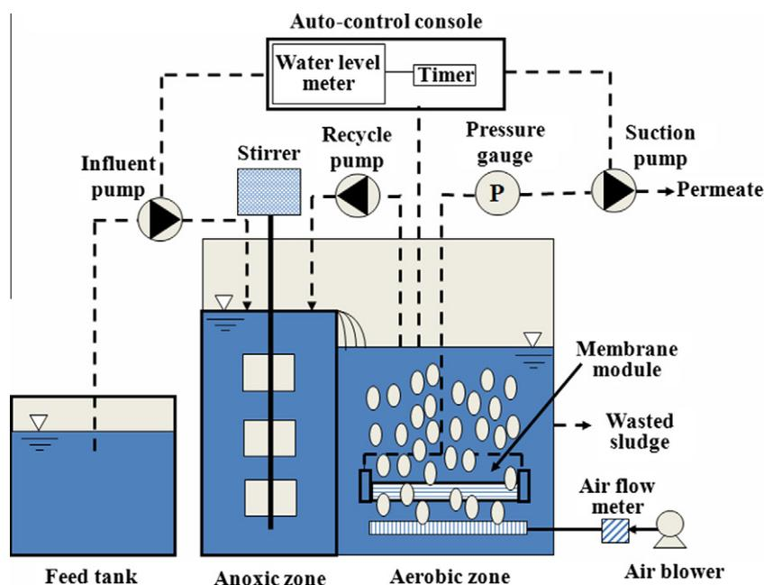
Fig. 1. Schematic structure of anoxic-oxic membrane bioreactor (A/O-MBR).
